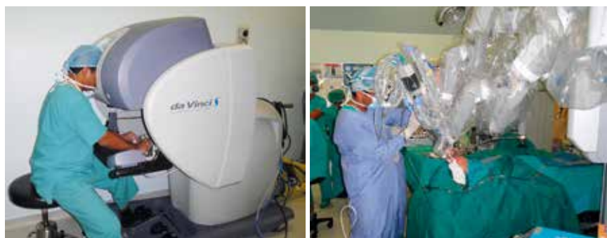
Figure 4. Trans-oral Robotic Surgery (TORS): The surgeon sits at a console and has high-definition 3-D vision of the operative field. The robotic arms enter the oropharynx and enable precise dissection of the tumour.
